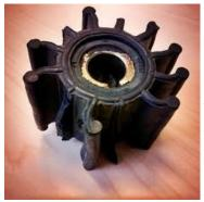
"set" that is normal. The rule of thumb is to replace the impeller if it shows signs of wear, has cracks between vanes or has missing or broken vanes. Also inspect the end plate and replace if excessive
