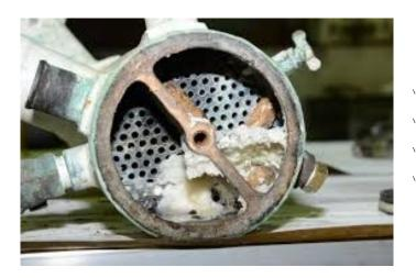
To completely remove particles from the heat exchanger, the circulation pump will need to be reversed pushing the solution backwards. During the circulation process the solution in the bucket will get darker as cleaning takes place. The solution will eventually stop cleaning as it is cleaning agent is consumed.
