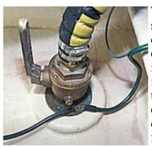
The seacock should periodically be exercised to prevent it from seizing in the open position. It can be extremely difficult to close a frozen seacock due to seizing.
